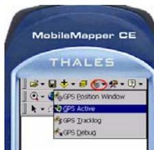
4. In the ArcPad tool bar, tap on the down arrow to the right of the Hammer/Wrench icon (
